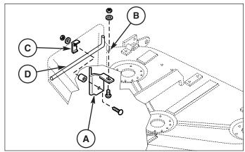
Figure 4. Install Discharge Baffle
